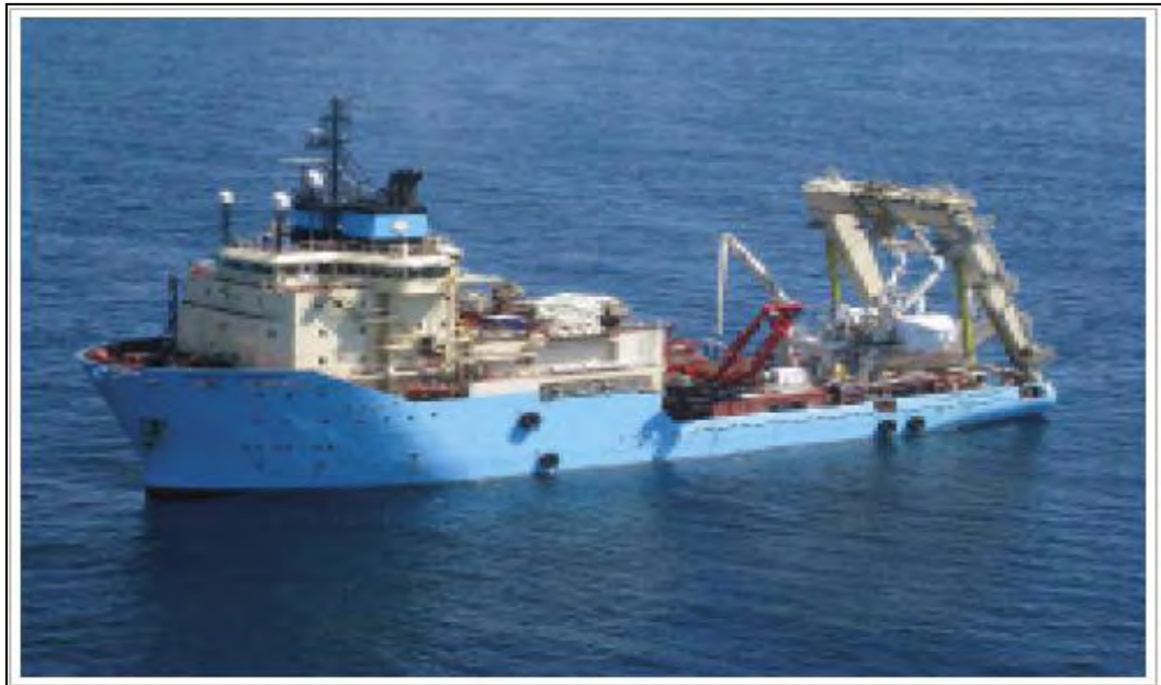
Figure 5-5: Cable Burial Vessel
