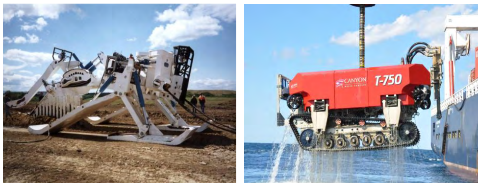
Figure 5-8: Installation Equipment: Cable Plough (left) Jetting Trencher (right)
