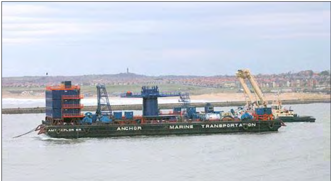
Figure 5-4: Cable Lay Barge
