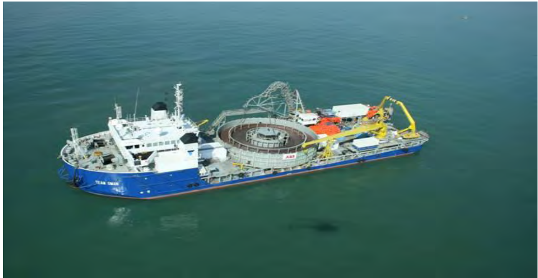
Figure 5-3: Cable Installation Vessel
